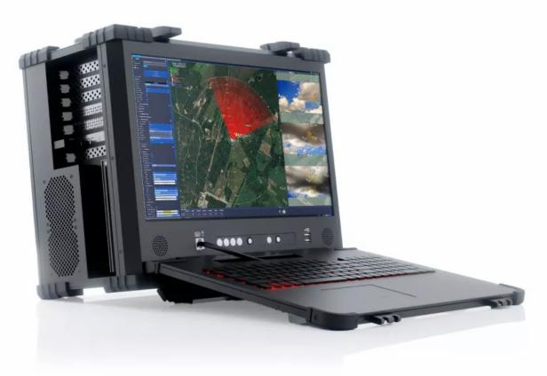
Compact, High Performance, Rugged Portable with a 17.3" or 18.5" display and 7 full-length expansion slots. Configurable with the latest Intel® Core™ or AMD processor.
